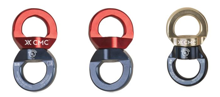
Our anodized aluminum swivels are available in two sizes to allow users to select the strength, weight and dimensions best suited to their specific needs. Whether used in a rescue haul system, helicopter operations, or rope access, the addition of a swivel can help prevent system lines from wrapping around each other, while at the same time reducing spin caused by loading a free-hanging rope.
